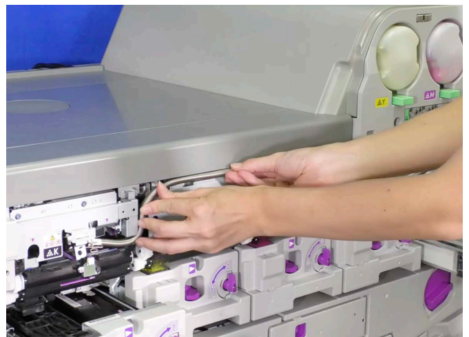
Carefully feed metal tubing for last position toner hopper along space provided as pictured.
