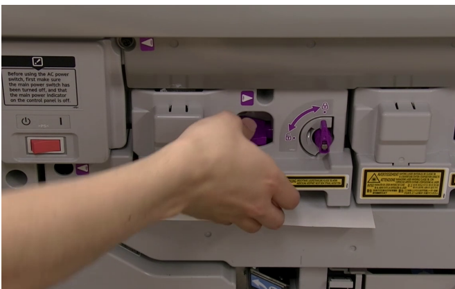
23. Carefully pull out White drum assembly from engine.
