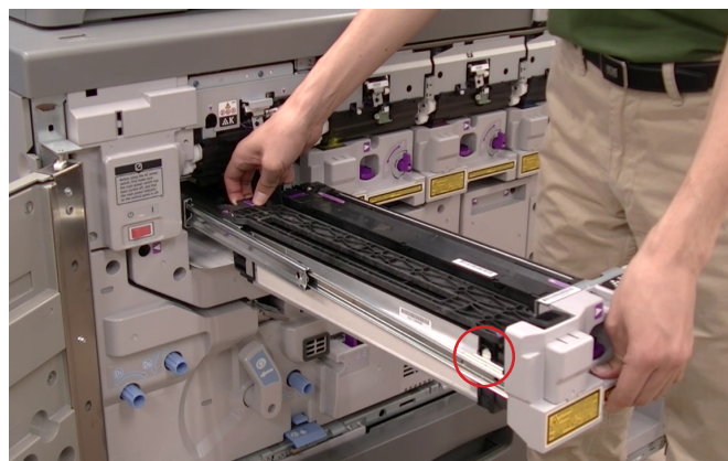
32. Carefully place on to rails, paying attention to holding pins (circled).
