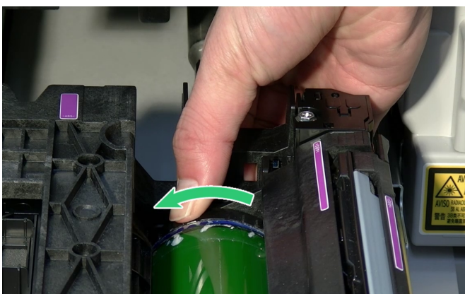
33. Carefully turn edge of drum till markings line up.
