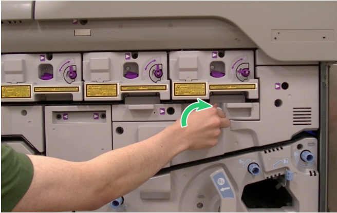
43. Turn latch to right and close front machine doors.
