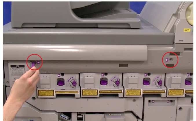
40. Replace screws holding upper cover in place.
