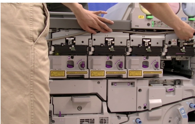
29. Feed spring tubing along path as pictured.
