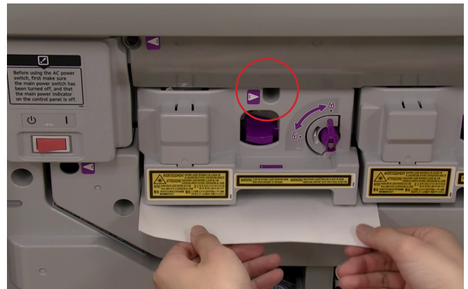
22. Place sheet of paper under White Drum assembly and remove screw (circled).
