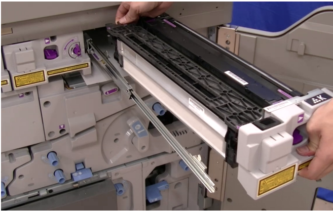
19. You may need to remove front locking screw and then carefully remove K drum assembly from rails.
