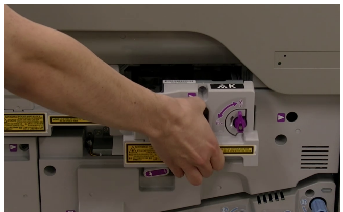
18. Press on release button and pull out drum assembly.
