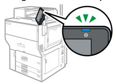
1. Open the cover of the main power switch on the left side of the machine, and push the switch.
